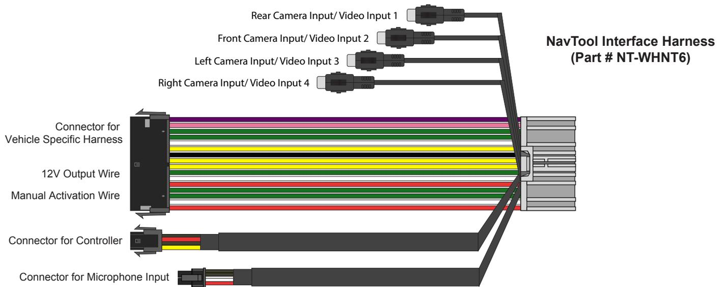
**Rear Camera Input /Video Input 1-** This input is dedicated for an aftermarket rearview camera or a video source with an RCA video output. Your vehicle factory camera will continue to work as before without any changes.
