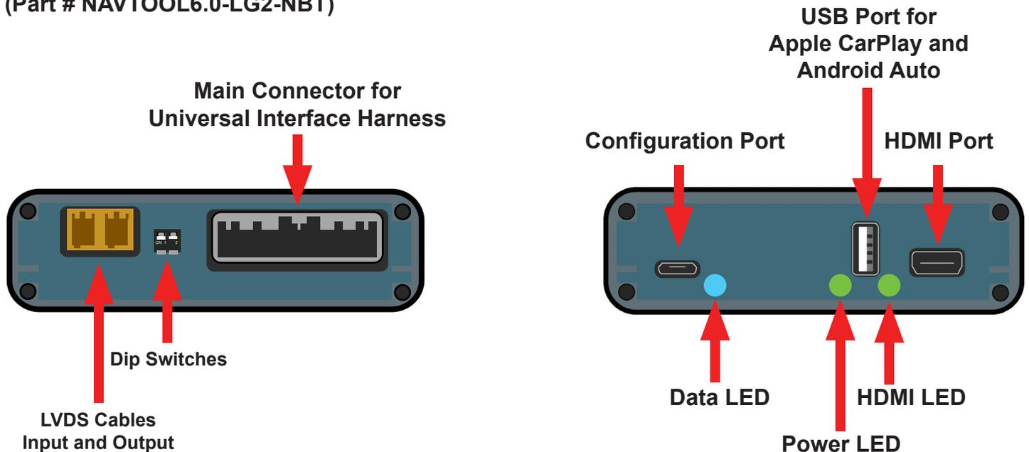
**Main Connector for Universal Interface Harness-** This port is dedicated for a connection of a universal wiring harness
