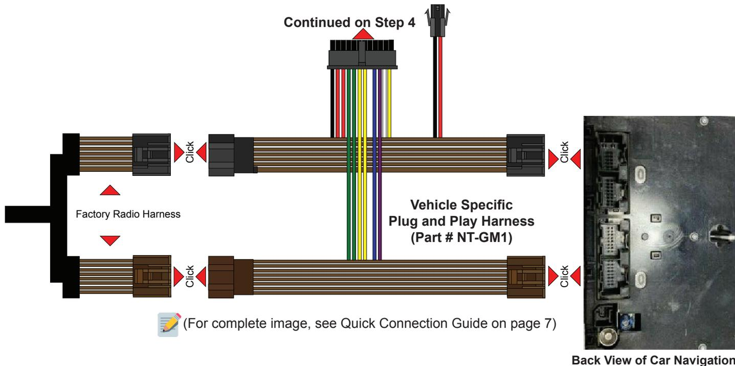
**Step 2:** ⚠️ Reconnect previously removed radio connectors into the back of the radio.
