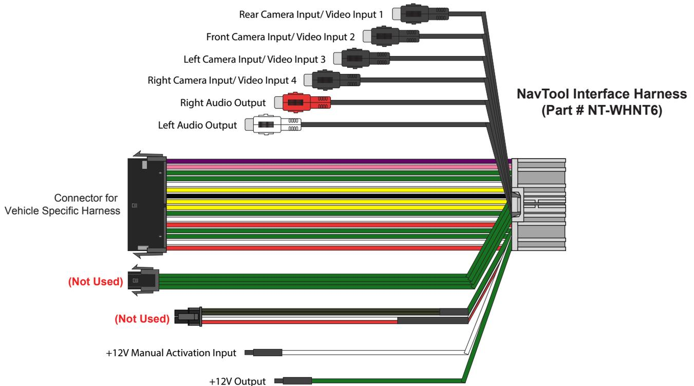
**Rear Camera Input /Video Input 1-** This input is dedicated for an aftermarket rearview camera or a video source with an RCA video output. Your vehicle factory camera will continue to work as before without any changes.
