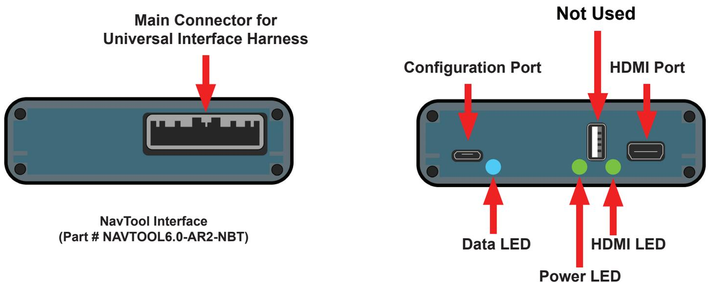
**Main Connector for Universal Interface Harness-** This port is dedicated for a connection of a universal wiring harness.
